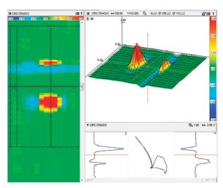
Circumferential cracks (75% and 50% at the support)
