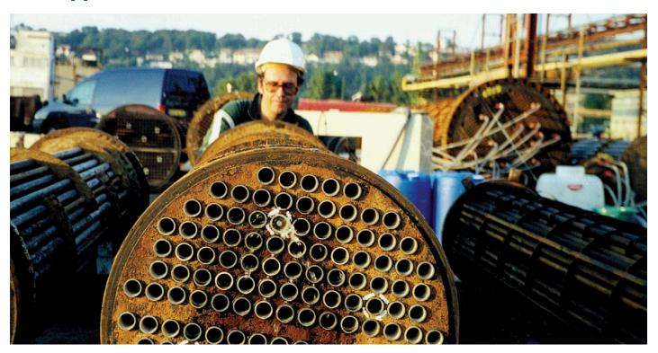
The internal rotary inspection system (IRIS) is an ultrasonic technique well suited to petrochemical and balance-of-plant (BOP) tube inspections. This technique uses an ultrasonic beam to scan the internal surface of the tube in helicoidal patterns, thus ensuring that the full length of the tube is tested. Olympus tube inspection systems monitor the front-wall and back-wall echoes to measure the tube wall thickness.
