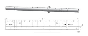
CT02 - ECT Extended ASME calibration tube.
