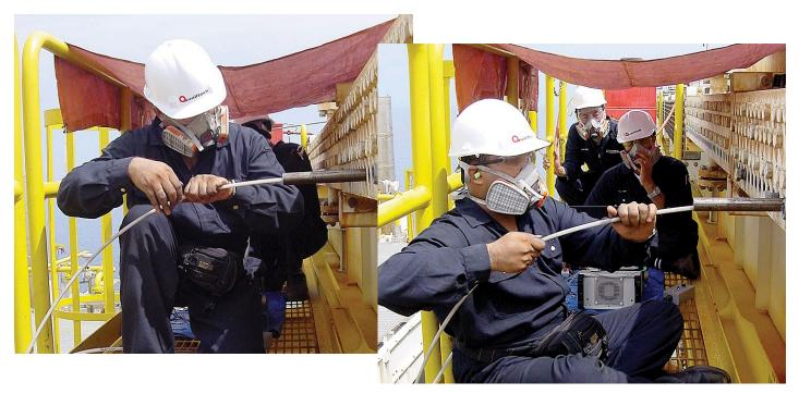
The magnetic flux leakage (MFL) technique is based on magnetization of the material being inspected. Magnetization is provided by a strong magnet located inside the probe. As the probe encounters a wall reduction or sharp discontinuity, the flux distribution varies around that area and is detected either with a Hall-effect transducer or an inductive pickup coil.
