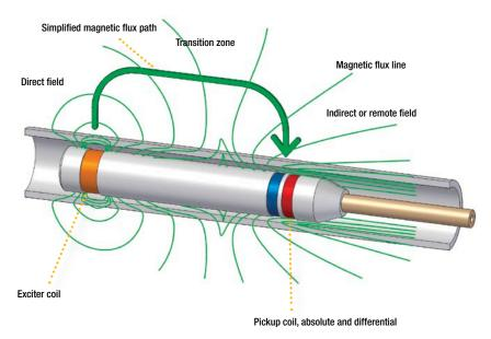
The distance between the pickup and exciter coils is 2.5 to 3 times the tube OD. (Single exciter model shown.)
